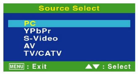
**Source Select:** To select an input source between **PC**, **YPbPr**, **S-Video**, **AV**, and **TV/CATV**.
